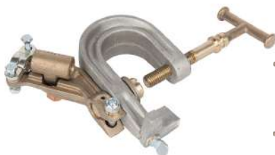
C6003598 Aluminum body and retainer, Bronze scrubber-type contact pads, Bronze T-handle with fine threads, Tapped for 5/8-11 UNC threaded ferrule
